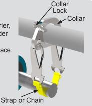
Vertical Cylinder Carousels can store multiple sizes and diameters of cylinders on a single system. Cylinders hang from the carousel carrier using a nylon/chain strap that is clipped to a cylinder collar. Multiple collars can be located anywhere on the carrier for various cylinder quantities and lengths up to the specified weight and off-balance limits of the carousel.
