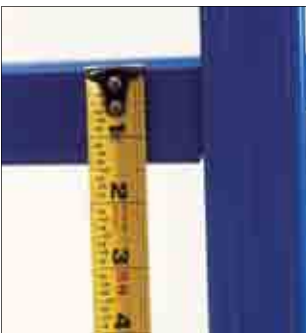
Low profile shelf beams are 1 1/2" high and adjustable on 1 1/2" centers.
