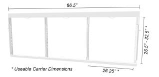
Each wire bay can be subdivided to accept a combination of spool diameters and sizes. For a combination of smaller spools, a spinner spool (Bay 2) may be used to best utilize the available cube.
