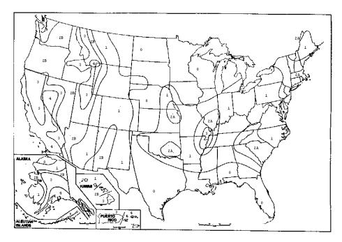
Zones 0 and 1 require minimal bracing and floor anchoring. Zones 2A through 4 require additional bracing and anchoring.
