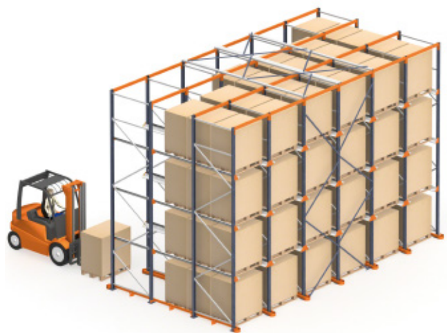
Figure 2: The stabilizing systems in Drive-In pallet rack include rigid frames, top tie beams with cross bracing and vertical cross bracing along the back of the system.
