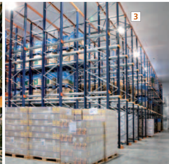
Freezer racking can store goods and single products for a long time.
