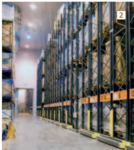
Half rotation orders or pallets of different sizes are stored on mobile bases.
