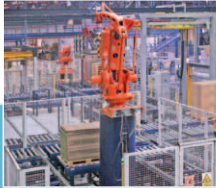
Automated picking with robot depalletizer
