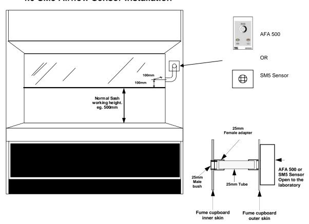
It is very important to position the AFA 500 or SM5 airflow sensor in the correct position to give long term stable reading of the face velocity. Please read the INSTALLATION NOTES below and if in doubt contact us for further advice.
