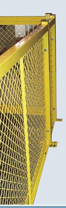
**PANELS:** Constructed standard with 10-gauge wire, woven in  $1\frac{1}{2}$ " diamond mesh &  $\frac{1}{4}$ " & 34" flat stiffener bars securely welded to 114" x  $1\frac{1}{4}$ " x  $\frac{1}{8}$ " angle frames with all joints welded. 3" x 1/8" steel kick-plate welded to bottom of panels. Panels come in 44" standard heights & equipped with slotted holes for quick mounting. 2" x 2" 14-gauge steel top rails are bolted to the top of each panel.
