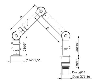
Part number: 70600344 Max. working radius: 630 mm (24,8 in) A: 400 mm (15,7 in) B: -
