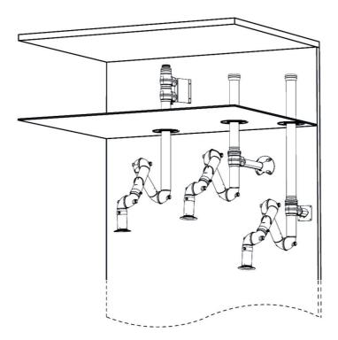
Wall mounting examples: Left: FX2-Up-PLUS arm with following accessories: -FX2-Wall-P BRKT kit-D-50/75/100-L190 -FX2-Ceiling cover plate-PLUS
