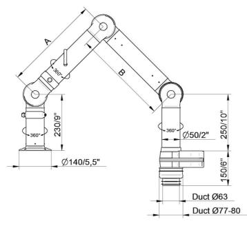
• FX2-ORIG-D50-L700-Up/Down-Low Part number: 70600144 Max. working radius: 630 mm (24,8 in) A: 400 mm (15,7 in) B: -
