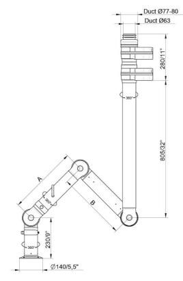
• FX2-ORIG-D50-L700-Up-PLUS Part number: 70600244 Max. working radius: 630 mm (24,8 inch) A: 400 mm (15,7 in) B: -
